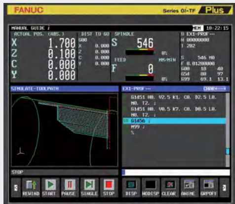
Check cutting path using cutting simulation
