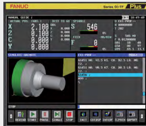
Check cutting result using cutting simulation
